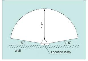
The location lamp has a high luminance with which the light from the lamp can be clearly visible at a position 10m apart from the location lamp along with a direction of an angle of 15° or more from the mounting surface.
